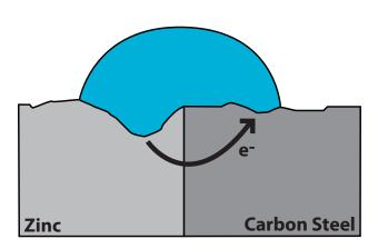
Figure 1 indicates how corrosion damages carbon steel. Note that the pitted area to the right is anodic and gives up electrons while the cathodic area to the left (where water and oxygen from the air are present) is where rust appears. The pitted area where the carbon steel is weakened is not where the rust appears.
